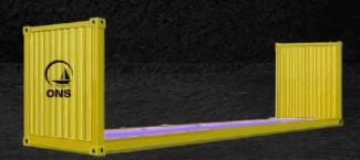
Open top containers are especially suitable for transporting overheight cargo, i.e. cargo taller than 2.54m (8'5"). They are available in two sizes: 20' and 40'. Cargo can be loaded by crane from the top-side. Over height cargo can also be loaded from the door-side since the door header can be swung open.
